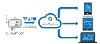
The GS1 continuously monitors environmental conditions and syncs the data to the UbiBot<sup>®</sup> IoT Platform. By offering 4 ways of data transmission, it can ensure different users access the online data using our App or the website.
